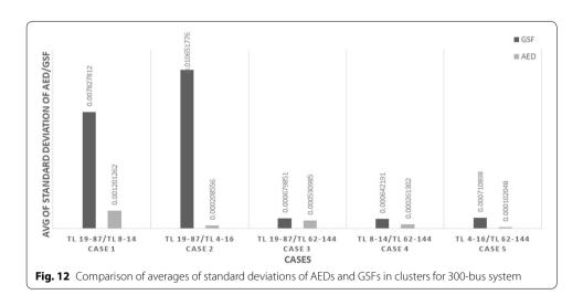
It can be observed from Fig. 12 that for each set of two tie-lines, buses in clusters created based on AEDs are more similar than those in clusters created based on GSFs since the average of standard deviations of AEDs in clusters for each set of two tie-lines is smaller than the average of standard deviations of corresponding GSFs. Based on the
