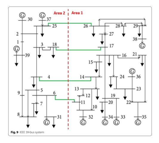
system to be divided into two areas interconnected with four tie-lines in order to analyse the impact of any injection change in generation/load zones on designated transmission line flows. In Fig. 9, area 1 comprises 24 buses, while area 2 consists of 15 buses. Bus 31 is chosen as slack bus.
