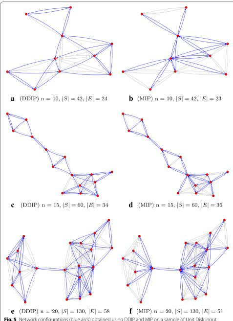
**Fig. 5** Network configurations (blue arcs) obtained using DDIP and MIP on a sample of Unit Disk input graphs: the output graphs with maximum possible efficiency,  $\mu$ , with a given limit on the number of active connections |E|. Gray arcs are the allowable arcs which were not used by a solution
