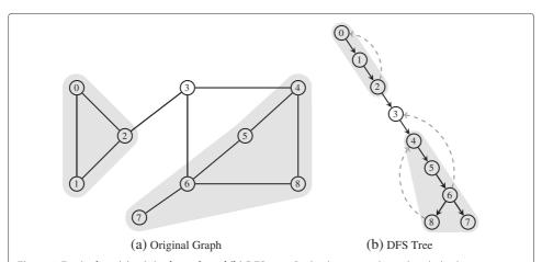
Figure 2 Equivalent (a) original graph and (b) DFS tree. Back edges are indicated as dashed arrows in DFS(0). The shaded areas correspond to resulting connected components if vertex v = 3 is removed from the graph. A traditional application of DFS is to detect cut vertices (i.e., articulation points), which forms the basis for our approach.
