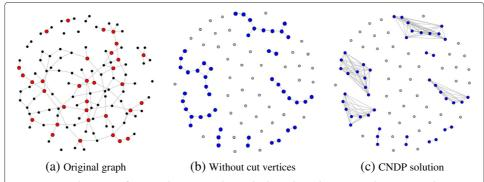
**Figure 1 Visualizations of an initial input graph, residual graph, and corresponding CNDP solution.**Visualizing an **(a)** initial input graph, the **(b)** residual graph after removing all cut vertices in the original graph (shown in red), and **(c)** the corresponding CNDP solution which highlights the fully connected subgraphs implied by Equation 1.
